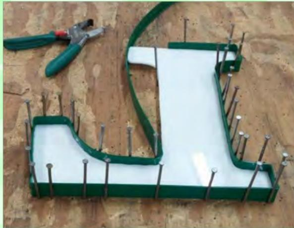
plexiglass to be attached to the sign cabinet. After gluing the Jewelite around the letters, it was secured by lining nails around it so the glue completely adhered to the edging. Once it dried, we replaced the newly fabricated letters on the sign.
